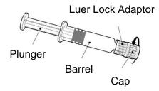
Hold the syringe by the barrel, not by the plunger.
